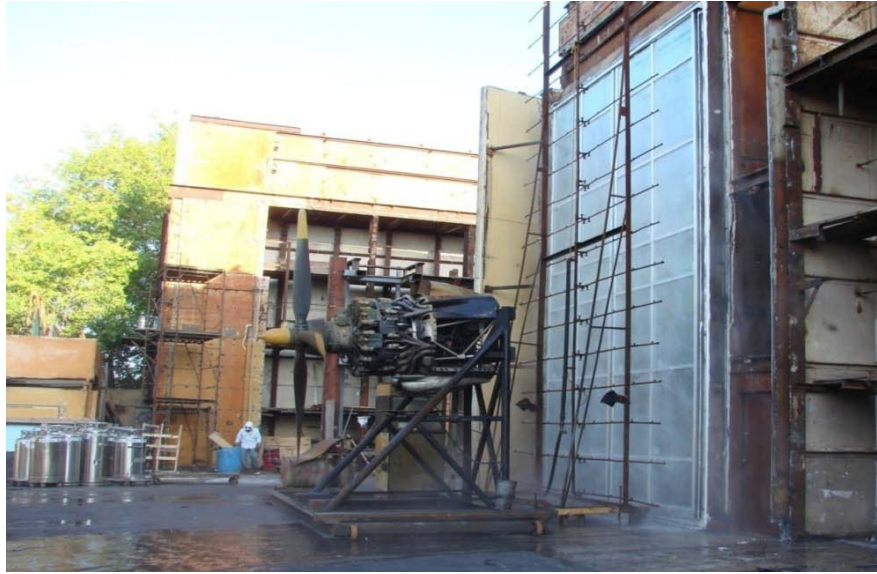
Figure 7. Dynamic water testing of a curtain wall in a laboratory. Only 5% of walls generally pass their first test.
